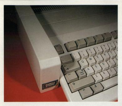
**LEFT: Datel's latest** ampling cartridge is different from other systems. Instead of using the Amiga's parallel port, the sampler plugs into the A500 expansion port.
